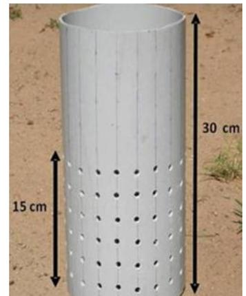
Field water tube made up of PVC.
